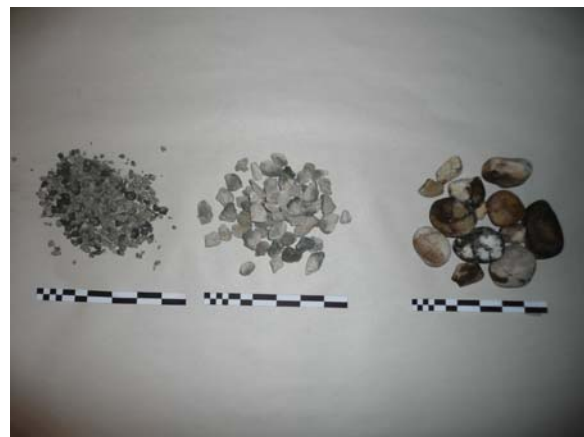
Figure 10: Aggregate varied in average diameter between <math>\frac{1}{2}</math> inch and 1½ inch. Most roofs had Size 67 (nominally ½” diameter).
